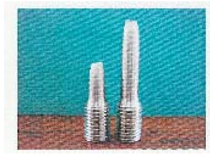
Tensile test of SUS-Ti junction by HIP
