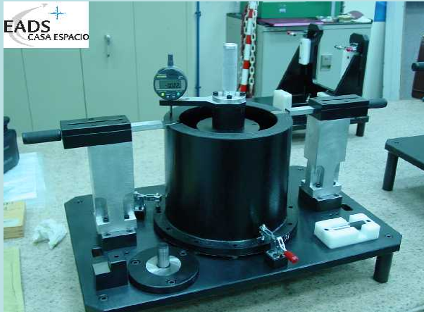
Dimensional control of columns with go/no-go gauges
