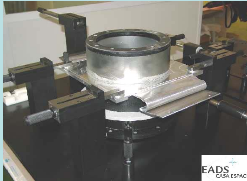
Dimensional control of complete support with go/no-go gauges
