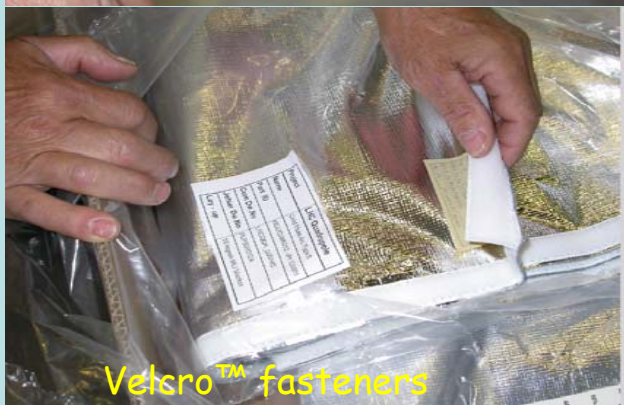
Interleaved reflectors and spacers
