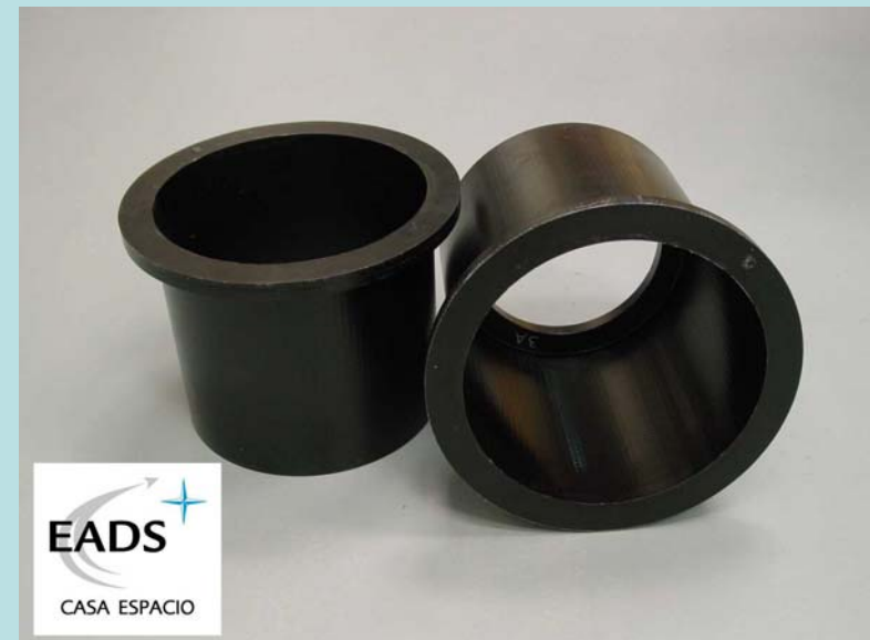
Columns as de-moulded
