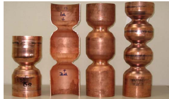
Formed Cu cavity test pieces
