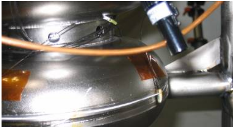
4 thermometers along equator EBW of cell#6
