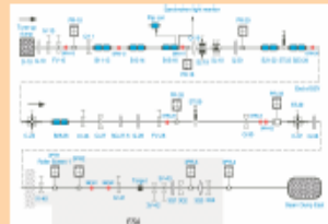
Fig. 2: A-Line from the Tune-up dump in the Beam Switchyard at the end of the Linac to End Station A. Downstream of IV-40 the beamline elements used for E158 (shown in Figure) have been removed in preparation for the ILC tests.
