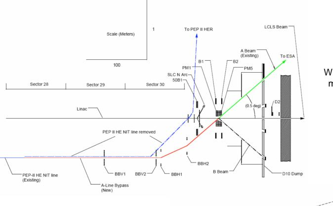
Will re-use PEP-II HE NIT line, modified to connect to A-line in the Beam Switch Yard
