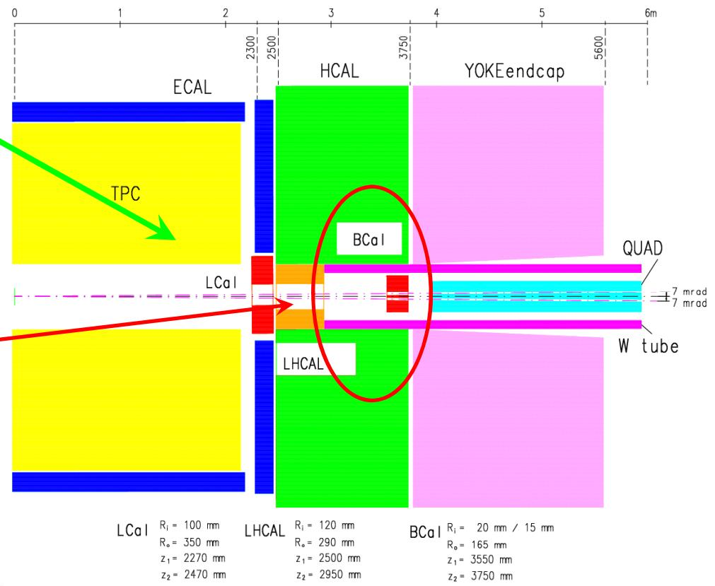
BeamCal will be hit by a large amount of electron-positron pairs stemming from beamstrahlung.
