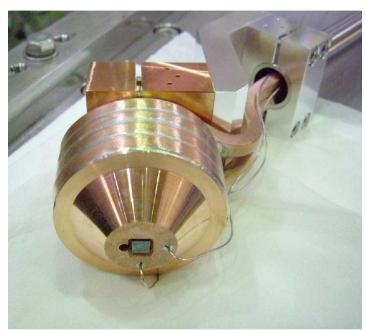
crystal tungsten (made in Russia) No. 1014 | 03L connected by HIP process (hot iso-static pressing)
