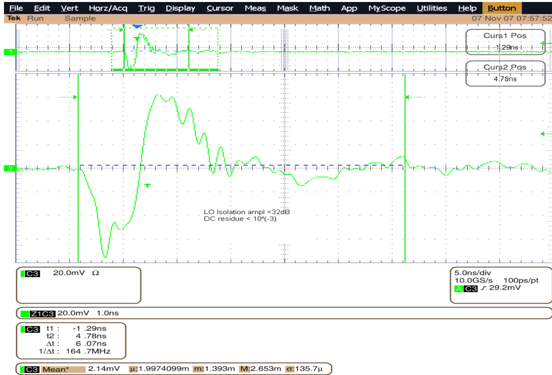
Fig. 3. LO p-t-p= \pm 1.6 V as in Fig. 2. The input=0. The LO p-t-p isolation is better than 32dB.
