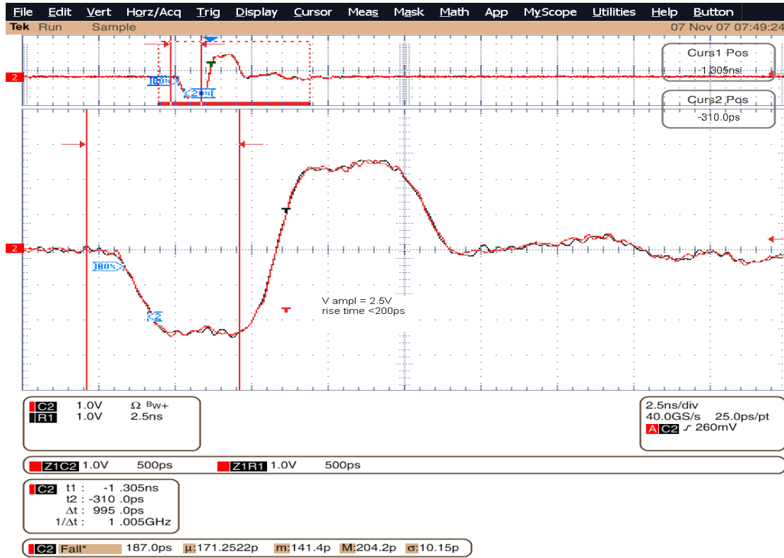
Fig.4. A SD CLOCK for in-time-multiplexing BPM. The SD clock (amplified by one or another RF2360 amplifier) is shown red and black. The amplitude is 2.4V. The fall/rise time is <200ps.
