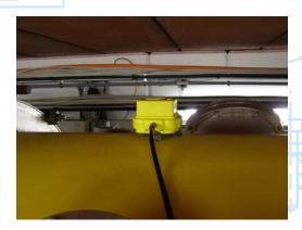
Triaxial sensor on vessel top
