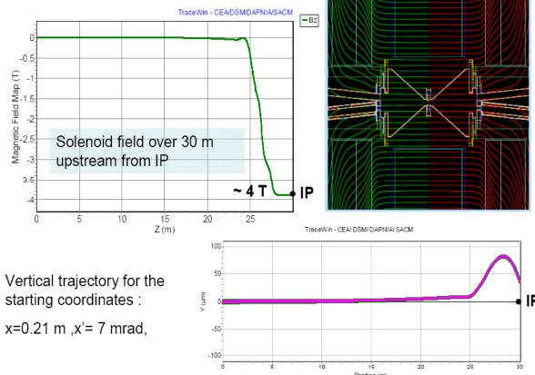
CEA-TRACEWIN calculation of the orbit deviation due to the solenoid
