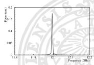
With a bandwidth of 50/300 MHz, the power coming from the NCR during the passage of a bunch train is 1.0/3.5 W.
