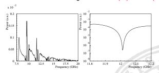
Minimum at 12 GHz: small transit time factor for the mode with m = n = 0 and q = 4, which has  $E_z(s) \propto e^{-s^2/2w_0^2}$ :
