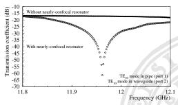
CST simulations show a clear rejection of the TE<sub>10</sub> mode of the pipe around the resonant frequency of the NCR.
