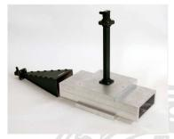
The horn antenna allows to inject TE and TM modes into the rectangular pipe.
