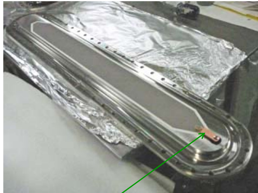
Connection between electrode and feed-through
