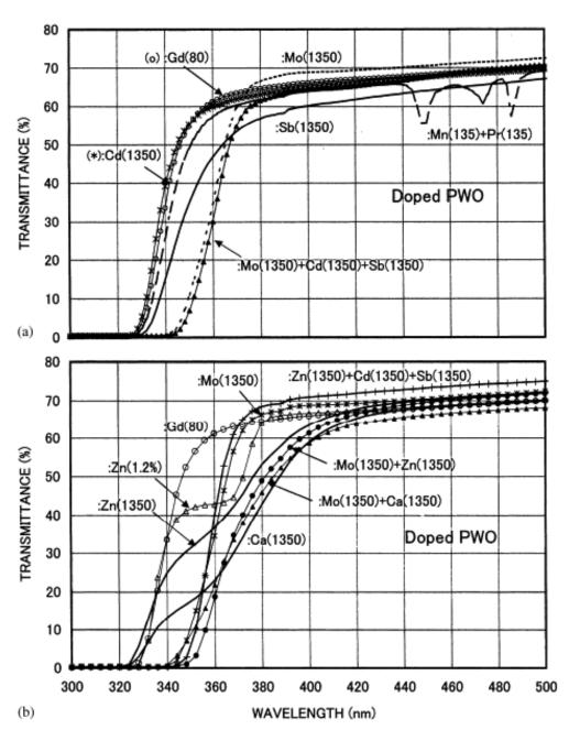
The transmission spectra of all kinds of doped PWO crystals are sufficient for transmitting Cherenkov light
