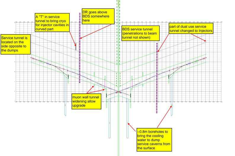
IR hall for push-pull, lengthened by 10m and deepened by 2m, with respect to Valencia, with two 16m shafts
