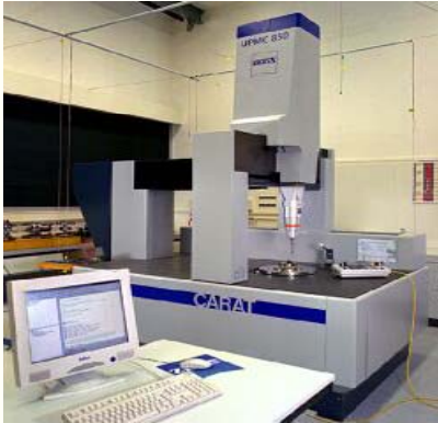
UPMC-850 CARAT S-ACCURATE CNC Range X: 850 mm Y: 1150 mm Z: 600 mm
