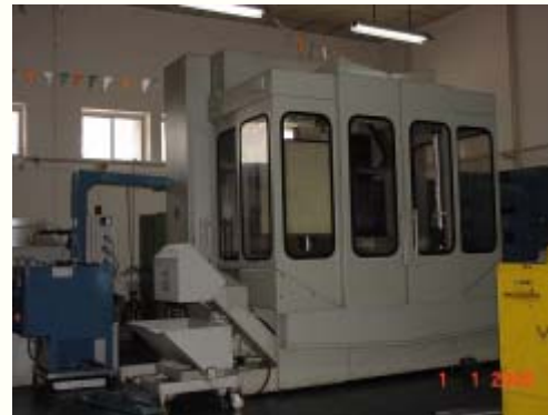
CNC VERTICAL BORING & MILLING CENTRE , Table Area:900X720 mm, Accuracy :0.005mm
