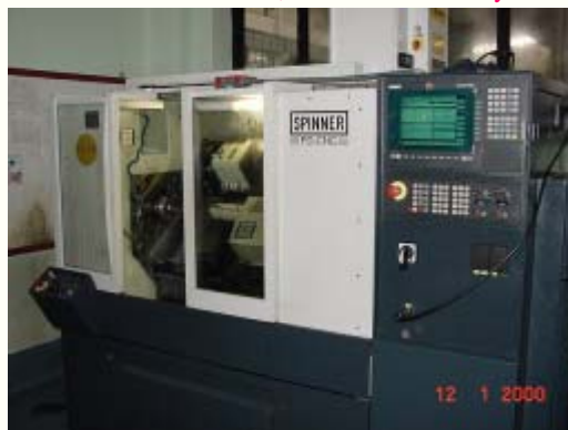
CNC, Ultra Precision Mount Bed Lathe, Length : 400 mm Accuracy : 0.002 mm
