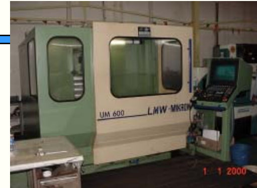
CNC Universal Boring And Milling Machine Table Area : 900X530 mm, Accuracy: 0.010 mm
