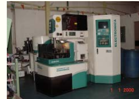
CNC Wire-Cut EDM Machine Super Cut 734 X: 250 mm, Y : 350, U&V : 73, Accuracy :0.010 mm
