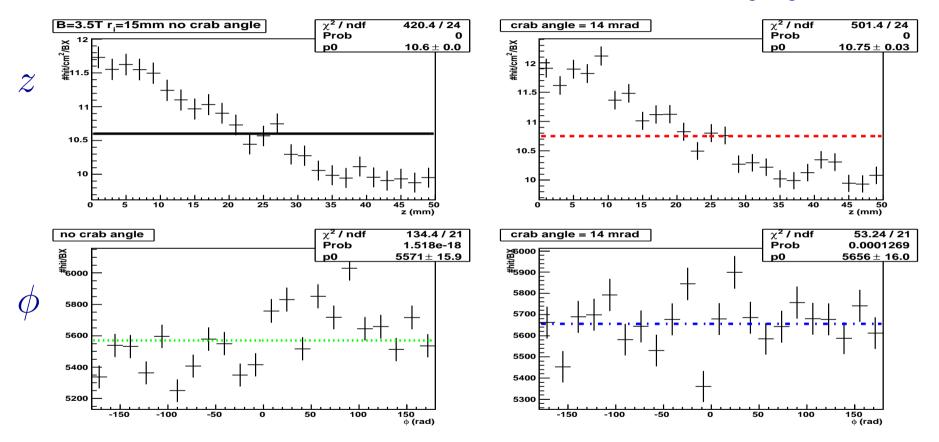
**Distributions in**  $\phi$  and  $z \Rightarrow$  no significant change between head-on & 14 mrad Xing angle distributions
