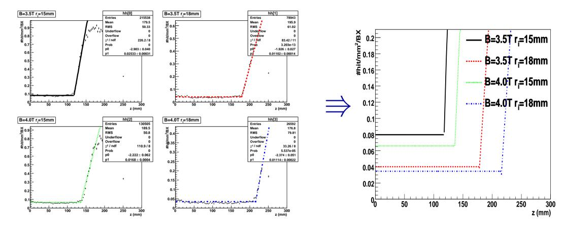
$\Rightarrow$  Use the corner between direct and defocussed  $e_{BS}^{\pm}$  to determine ladder lengths  $\rightarrow$  angular coverage
