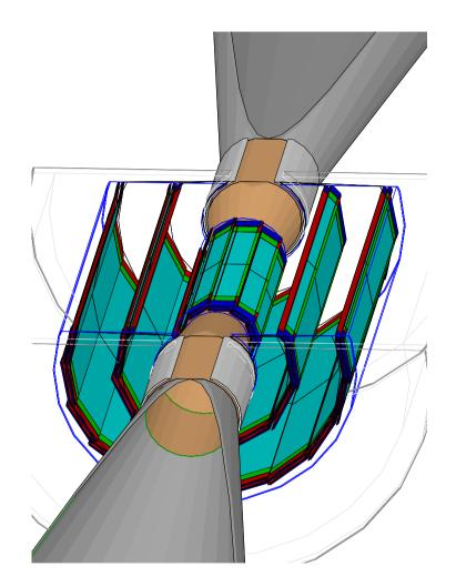
Ladder geometry  $\rightarrow$  accommodate simultaneously different sensor technologies :
