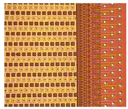
High speed (busline-free) devices with 2level metal clock distribution:
