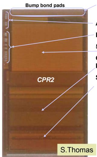
Wire/Bump bond pads Voltage and charge amplifiers 125 channels each Analogue test I/O Digital test I/O 5-bit flash ADCs on 20 µm pitch Cluster finding logic (2×2 kernel) Sparse readout circuitry FIFO
