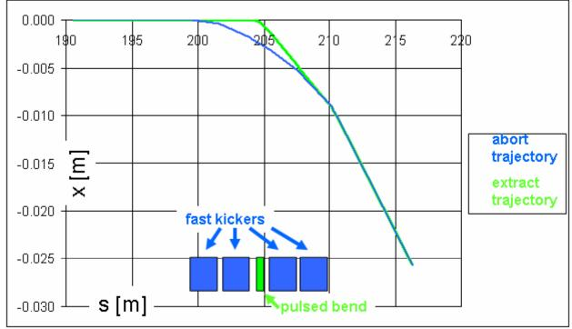
The ELBC2 extraction system consists of ten 1m long fast abort kickers, and a single 1m long tune-up extraction bend placed in between two central kickers. The abort kickers can be charged to 90G each in 100ns. The tune-up bend is excited to 900G.
