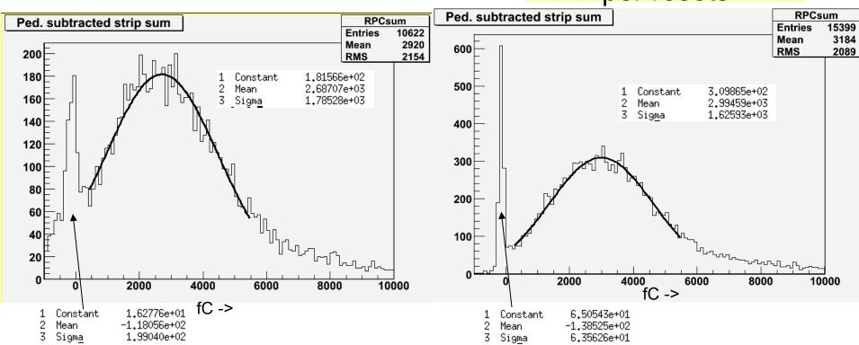
In normal LC operation the KPIX charge amp is reset between beam pulses every 400ns A continuous DC reset mode was added for cosmic rays tests However, the noise seems 2-3 times worse in DC mode Noise 8 times worse with no reset
