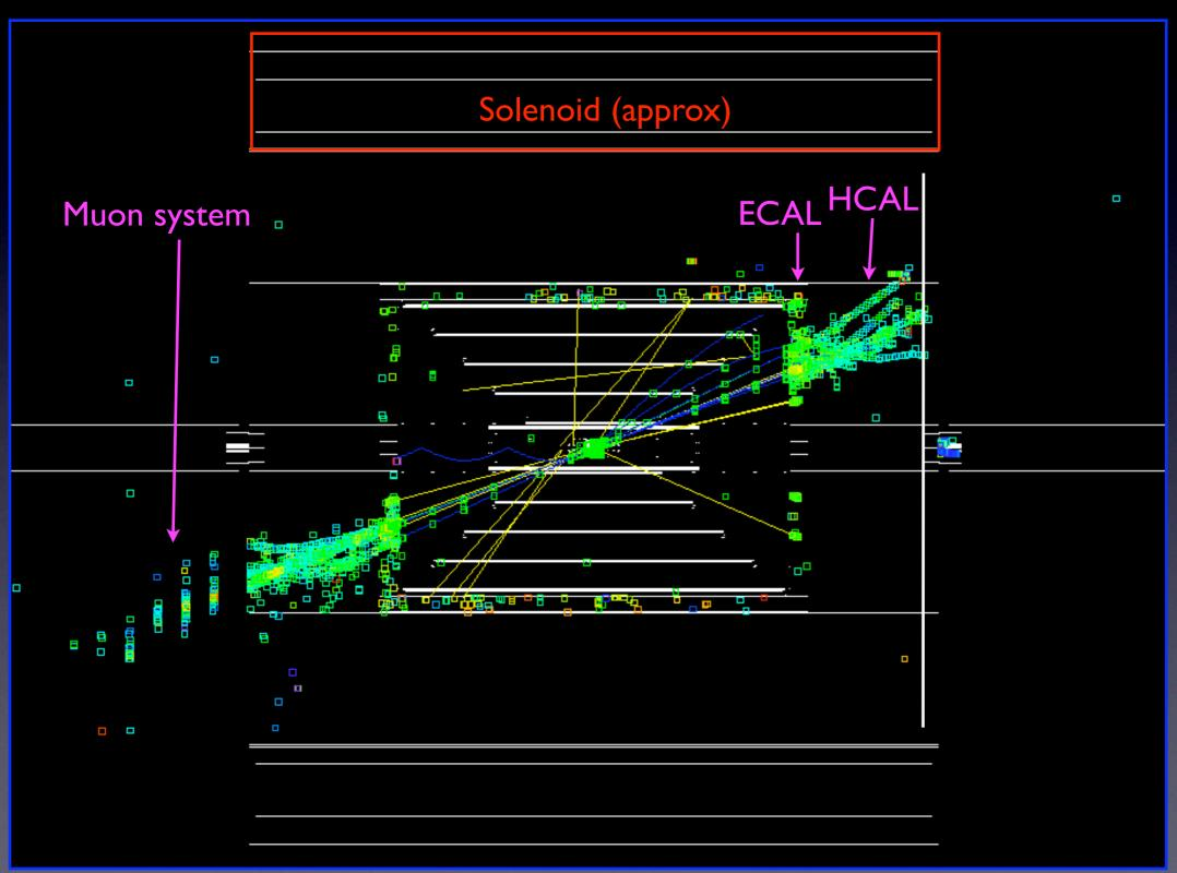
This is with the sid02 muon system (20cm steel plates).
