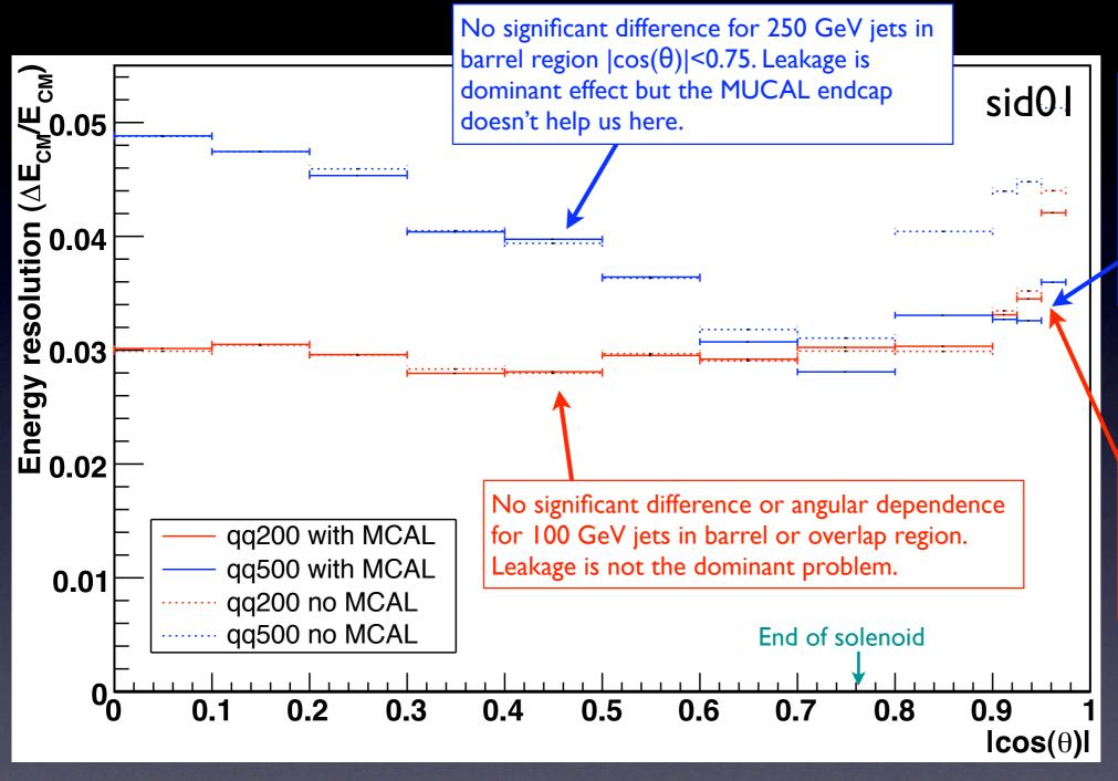
Big improvement for 250 GeV jets in overlap/endcap region. MUCAL solves the leakage problem and makes endcap resolution much better than barrel. Acceptance dominates at very small angles
