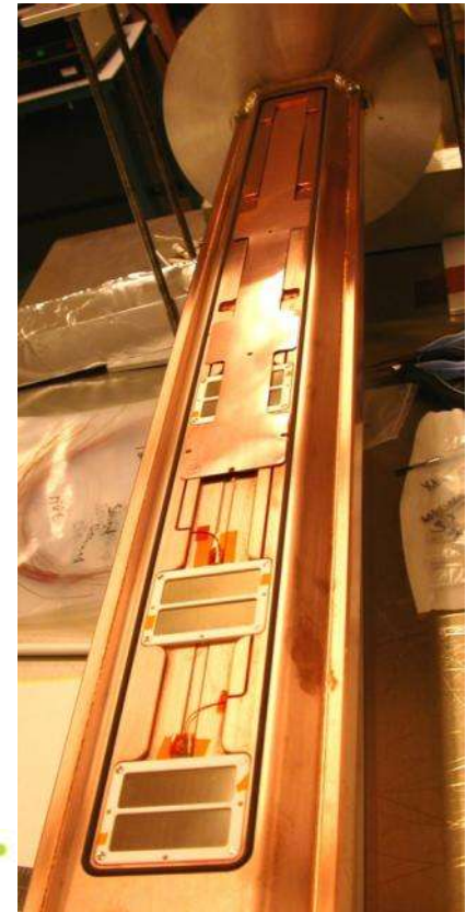
Retarding field analysers for electron cloud measurements in wiggler chambers.
