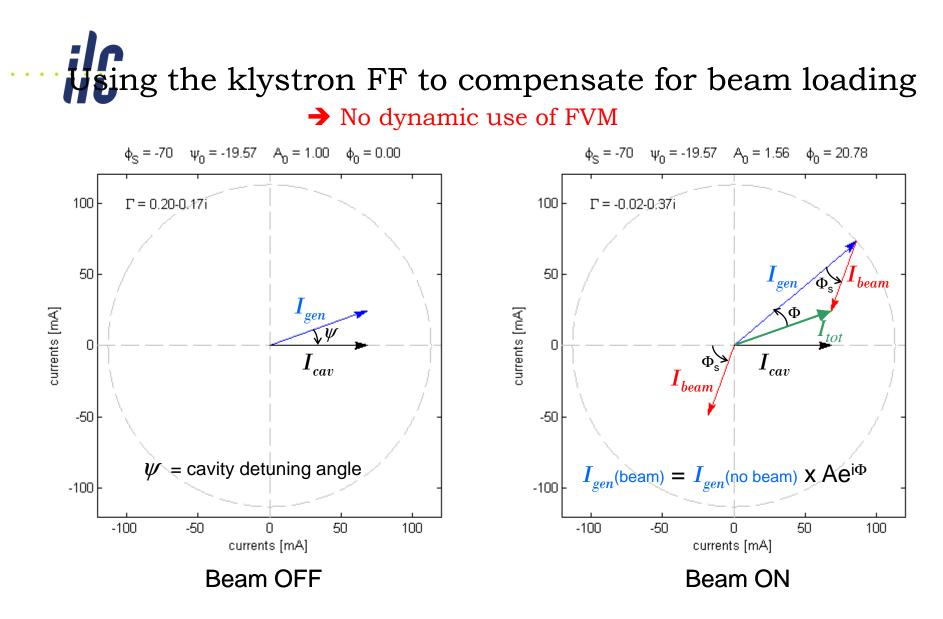
Assuming nominal beam loading, there is no need to modulate the klystron forward power using the ferrite vector modulator if  $I_{tot}(\text{beam OFF}) = I_{tot}(\text{beam ON})$
