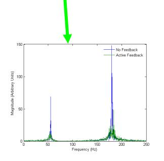
Matlab simulation of NBFB in CW cavity
