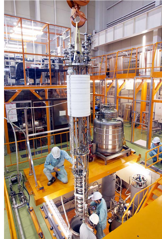
Installation test into cryostat
