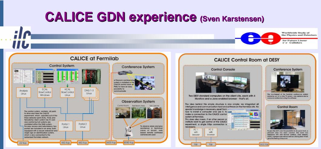
Remote operation of CALICE test beams at CERN and FNAL : dedicated ROC at DESY with : 2 PCs 4 screens each and a Video Confernecing system control via internet using : HTTP, Sun Secure Desktop communication via internet using ESnet and WEBcams with HTTP interface (remote controlled) Successfully used for Test beams Not shown at this workshop (but worth to note): CMS just finished 4 weeks of cosmic running with remote DQM shifts done from the CMS ROCs at CERN, FNAL and DESY
