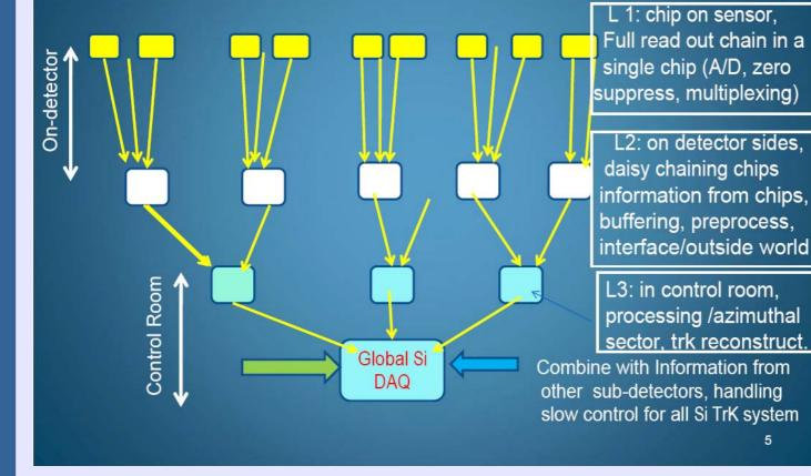
*3 Level DAQ approach* for silicon strip trackers
