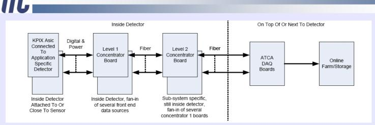
XPIX on or close to sensor L1 Control/Concentrator L2 Concentrator if needed ATCA based DAQ
