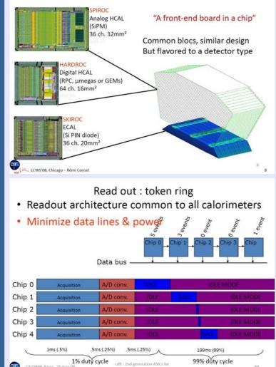
Getting very close to real design 3 different ROC designs for AHCAL, DHCAL, ECAL *Common readout architecture for all calorimeters*
