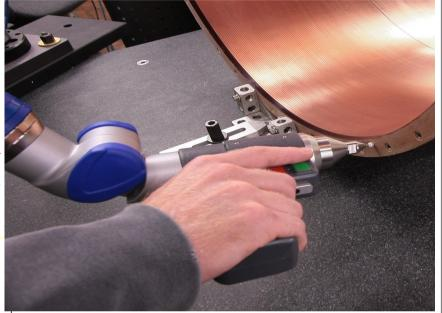
Intrinsic measurement precision per point: around 20 µm
