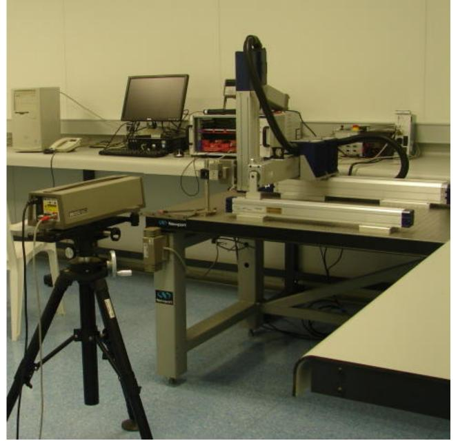
**Linearity** (comparison of reconstructed position of a fixed laser spot scanned over the sensor vs displacement of motors) will be studied using a 3D motion table.
