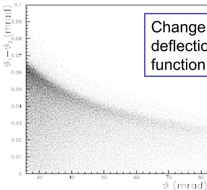
Change in the final state polar angle due to deflection by the opposite bunch, as a function of the production polar angle.
