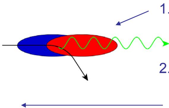
1. High beam-beam field ( $\sim kT$ ) results in energy loss in the form of synchrotron radiation (beamstrahlung).
