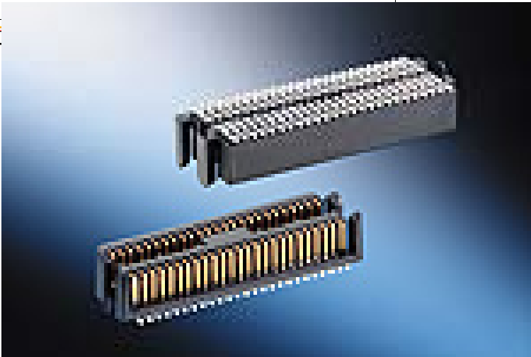
ERNI microstac 0.8 pitch, 50 pins
