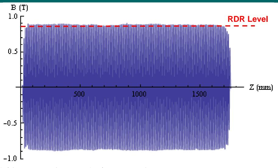
Field measured at nominal current of 215 A RDR Field level (0.86 T) achieved for the first time in a full length magnet (peak field is 0.88  $\pm$  0.014 T)
