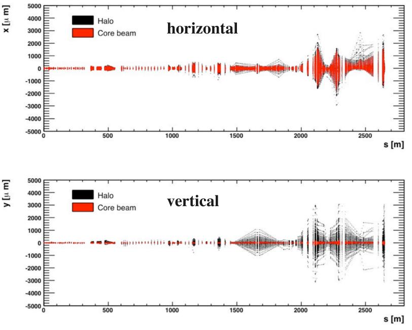
LINAC + BDS : fraction of 10<sup>-4</sup> of beam particles hit spoilers in ideal machine - no misalignment / errors
