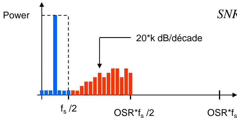
$$SNR_{dB} = 6.02N + 1.76 + 10 \log \left( \frac{2k+1}{\pi^{2k}} \right) + 10(2k+1) \log(OSR)$$
