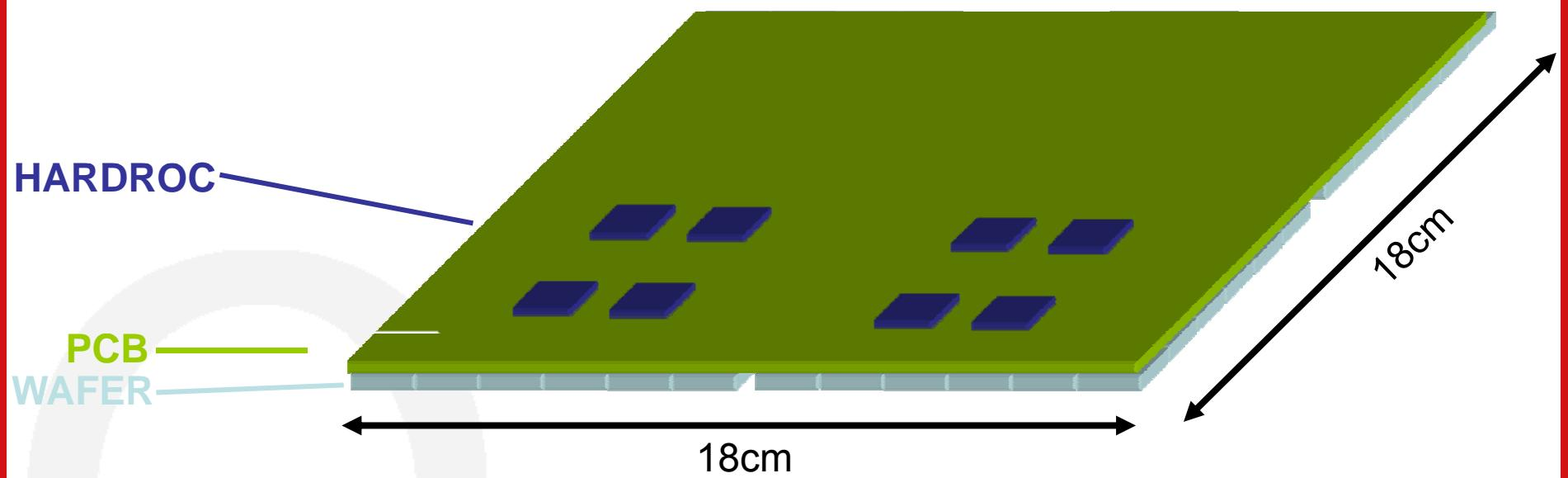
1296 channels. 8 HARDROC (512 channels equipped)
