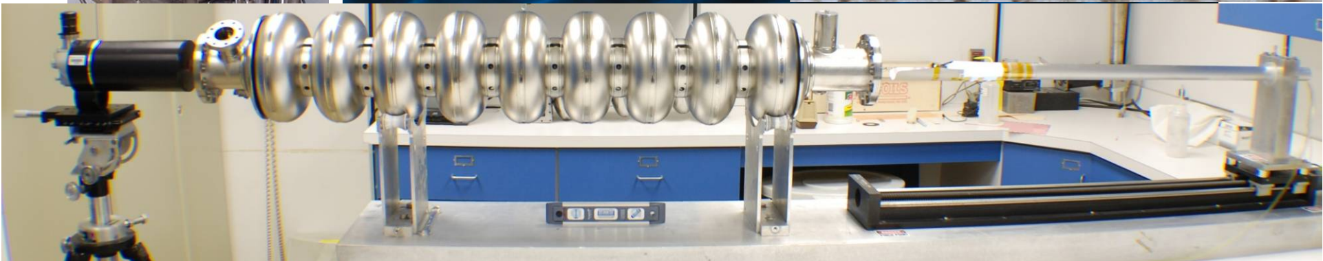
High E field region AES4 - Field emission limited
