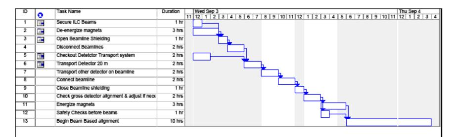
With careful engineering and an experienced, well rehearsed crew, it seems plausible to make the push-pull cycle, not including the beam based alignment and re-tuning of the machine, in less than a day.
