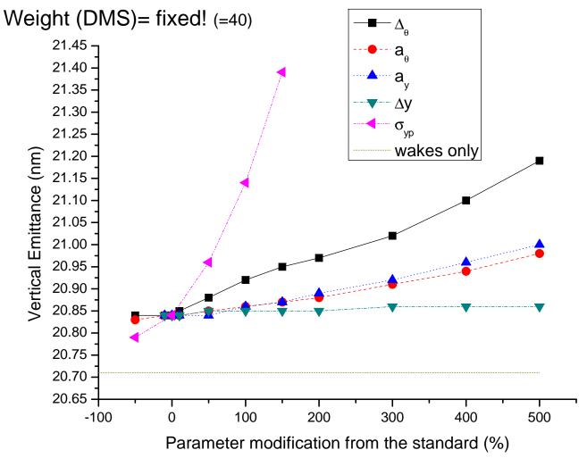
The model here only uses the correction as given in the version 0.7 of the misalignment paper. Emittance (or  $\epsilon_{yc}$ ) here is the vertical emittance with the energy correlation numerically removed
