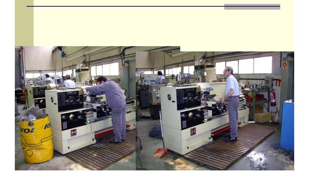
2 parallels torn of aprox diam 0.2x0.6 m. Accuracy of aprox 0.03 mm/m, with temperature compensation.
