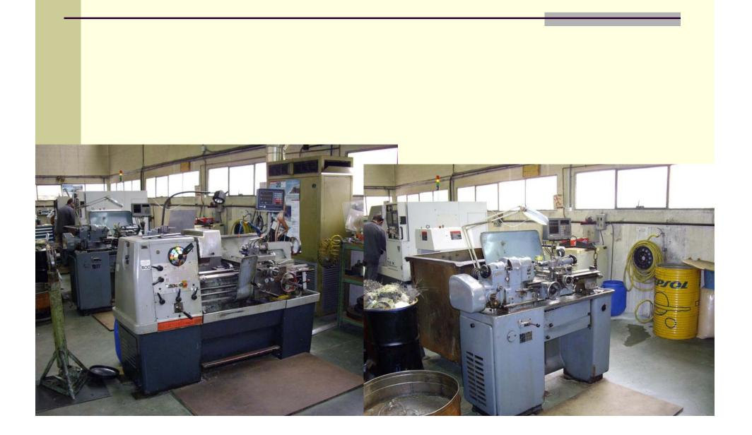
1 parallels torn of aprox diam 1x2 m. Accuracy of aprox 0.04 mm/m, with temperature compensation.
