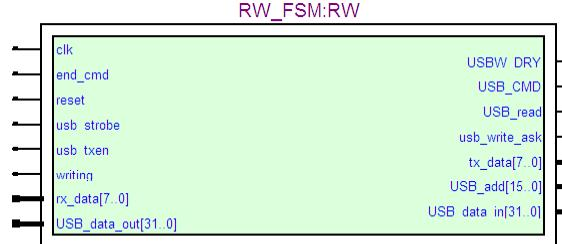
SM which determines if USB accesses are registers access (16 bit address, 32 bit data) or commands
