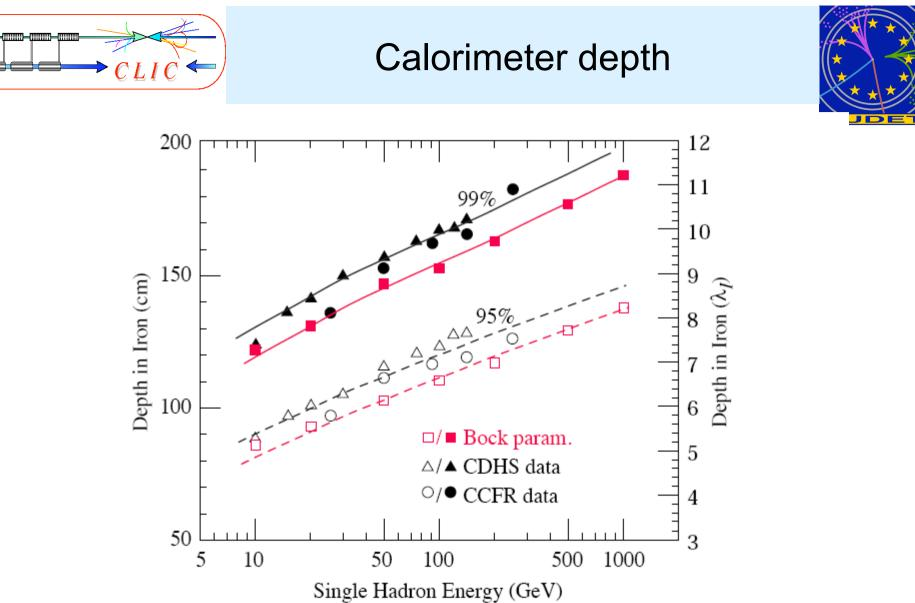
Figure 28.22: Required calorimeter thickness for 95% and 99% hadronic cascade containment in iron, on the basis of data from two large neutrino detectors and Bock's parameterization [143].
