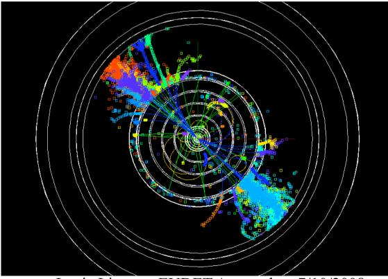
3 TeV e<sup>+</sup>e<sup>-</sup> event on SiD detector layout, illustrating the need for deeper calorimetry
