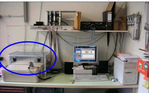
in the LPTPC setup the signals have to be delivered to the readout electronics via 2 m long twisted pair cables (adapter cards had to be designed)
