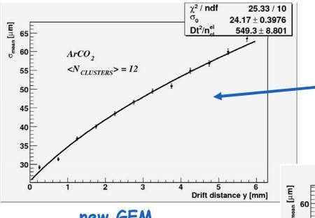
old GEM configuration with 120  $\mu$ m projected z-pitch
