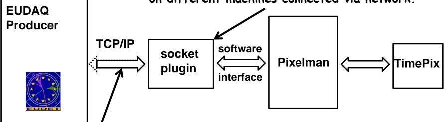
As an option / Pixelman can also send commands to the DAQ via the socket plug-in
