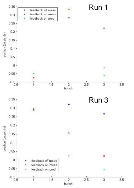
Run1 – bunch3 position seems to have changed relative to bunch1 and bunch2. Gain appears to be correct
