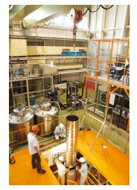
magnetic shield was delivered in July 14. It was already installed. (residual field ~50mG) The next V.T. of AES001 is scheduled in Aug. 25-29
