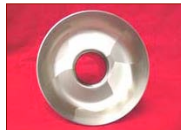
Fig. 5. Inner surface of a large grain cavity at JLab.
