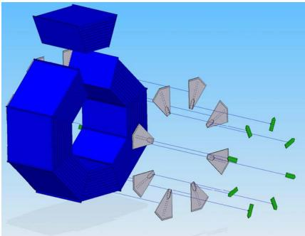
Ecal and Hcal : mechanical design straightforward scales for a longer barrel Longer Ecal Kapton cable, larger GEM-µMega-scintillators
