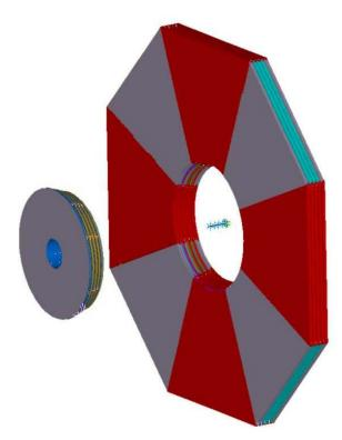
Very rough estimate of bending assuming central force of 5000t and unsupported diameter of 8m: 10 mm
