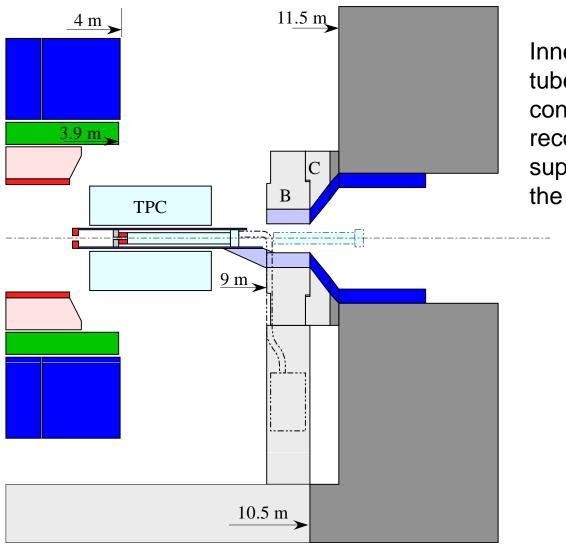
Inner-tracker support tube is usually connected toTPC, and reconnected to QD0 support tube during the maintenance
