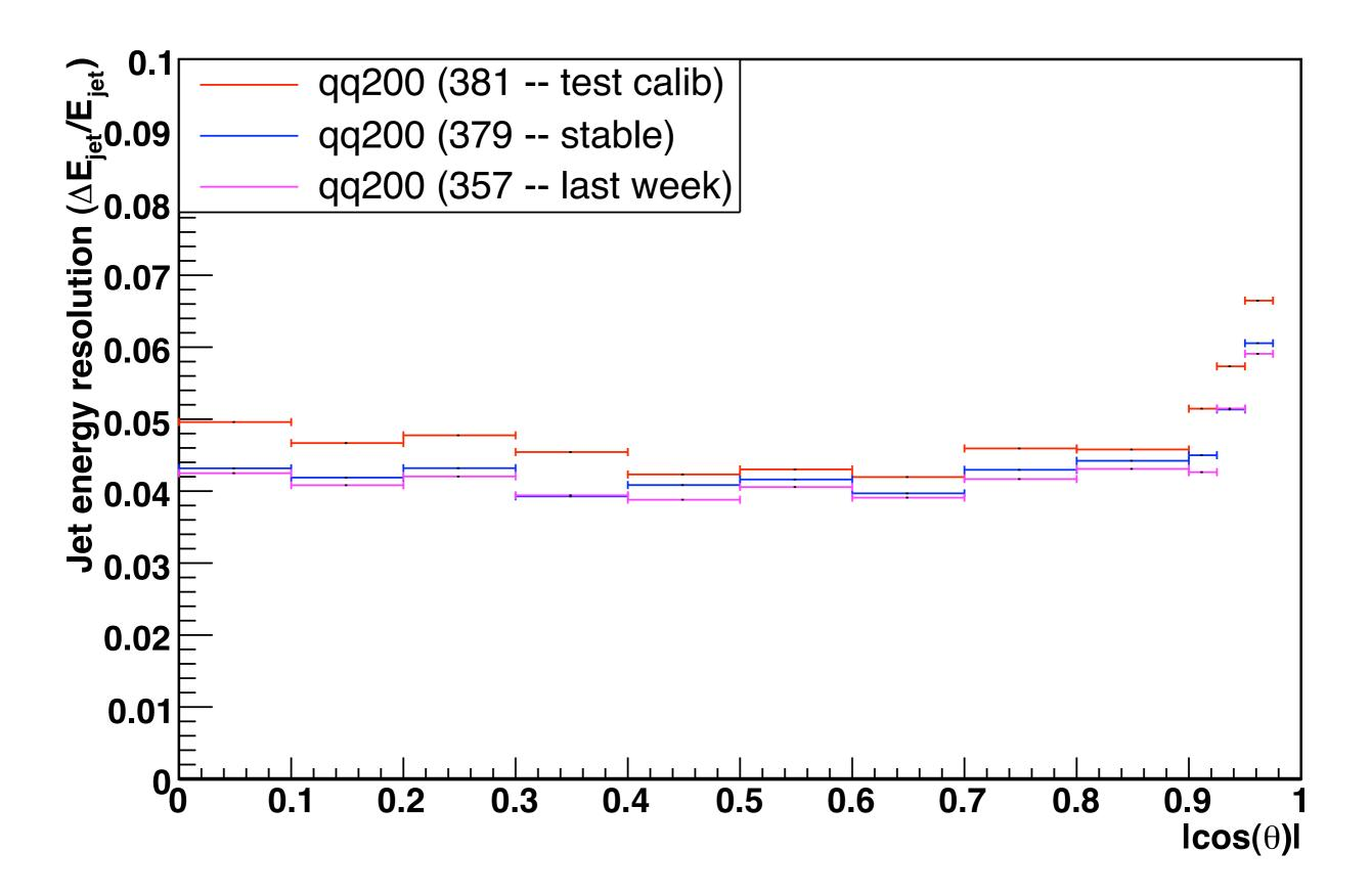
For 100 GeV jets, test calibration is worse (as expected).
