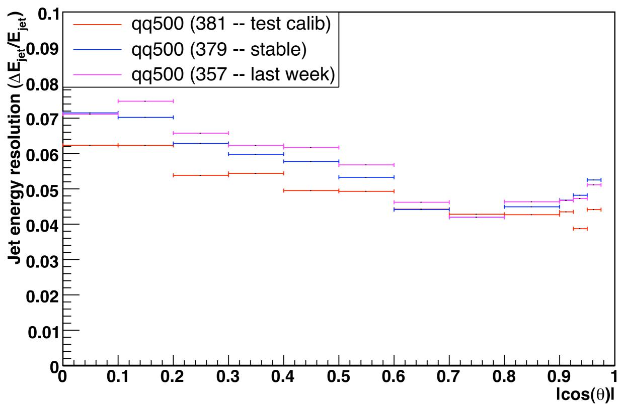
For 250 GeV jets, test calibration improves pretty significantly. Barrel performance surprisingly good -- not fully understood, but a clear pointer that we have potential to improve resolution here.
