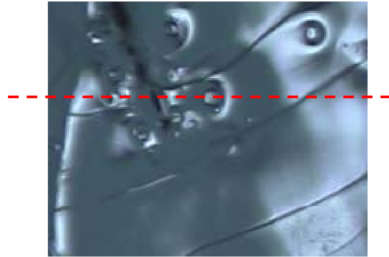
#6 cell equator, Z = 734 mm, t = 199 deg. heating spot
